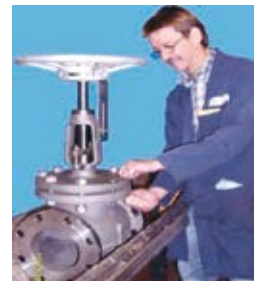
All valves are assembled and quality checked prior to testing.
