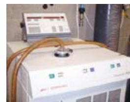
Emission Tests are conducted via Maspectrometer Leak detector
